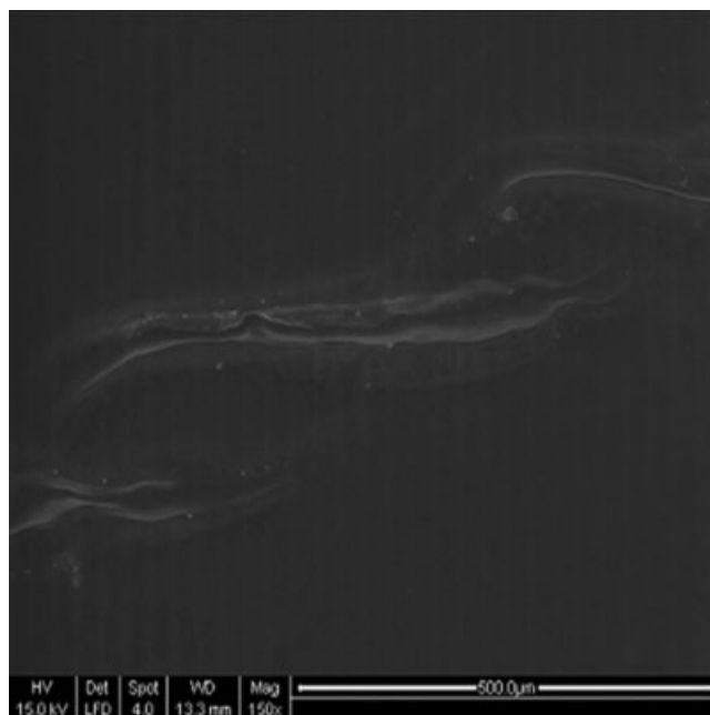
Figure 12 SEM image of the crack propagation in the optimized model.
